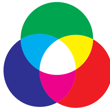
FIGURE 2 Additive color mixing. Simulated overlap of projected red, green, and blue lights. The additive combination of red and green is seen as yellow, red and blue as purple, green and blue as cyan, and red, green, and blue as white.
